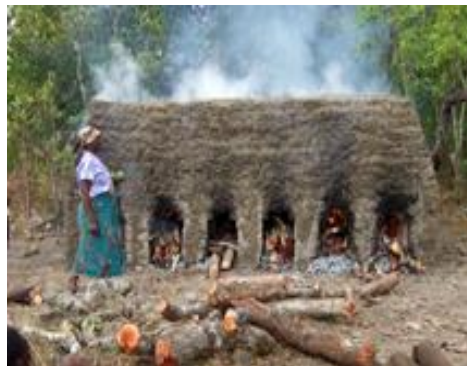
A firewood-based conventional brick kiln
