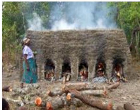
A firewood-based conventional brick kiln
